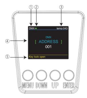
1. DMX means the light is in the DMX mode.Similarly,SLAVE means the light is in the SLAVE mode.
