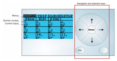
Figure 1: LCD main screen and buttons for navigation and programming
