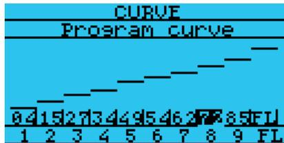
Figure 6: Each programmable curve has ten steps.
