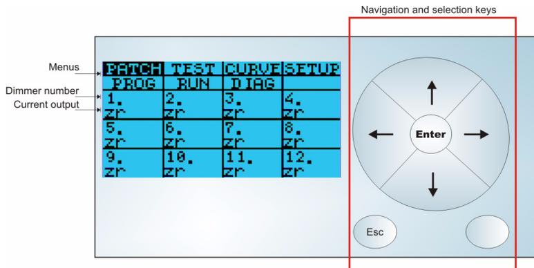
Figure 1: LCD main screen and buttons for navigation and programming
