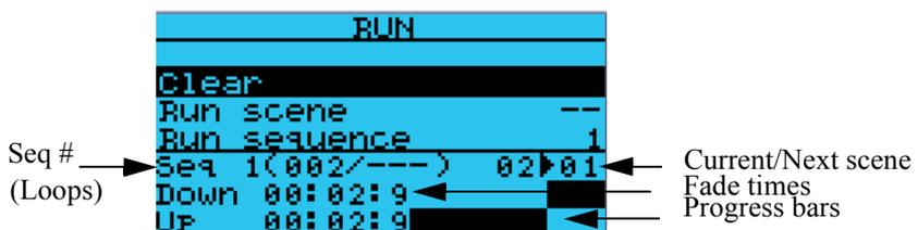
Figure 13: The Run screen with sequence details
