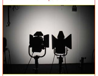
The Beam in full flood is NARROW (only 45°) and shows an HOT SPOT (large area to go from Beam to Field Angle) LED FIXTURE by "DE SISTI" EXACT FRESNEL performances
