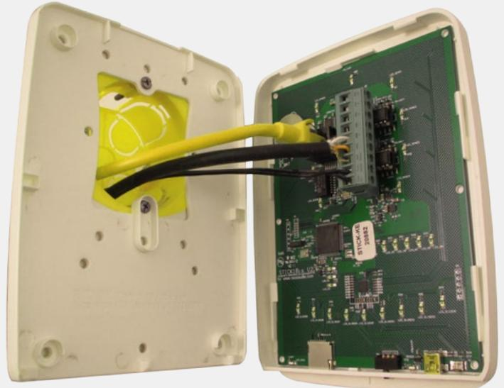
**\*\*CHECK PIN CONFIGURATIONS. APPLYING POWER TO THE DMX INPUT WILL DAMAGE THE CONTROLLER\*\***
