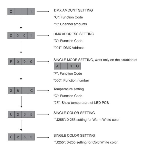
Press the "MODE" then press the "ENTER" to begin your setting. Press "UP" and "DOWN" to switch the modes with the shining Function Code. Be sure to press the "ENTER" button to save your changing, it won't be saved if the button has not been pressed. Moreover, the saving data still exists even after power off and then on.
