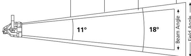
For Field diameter at any distance, multiply distance by 0.32
