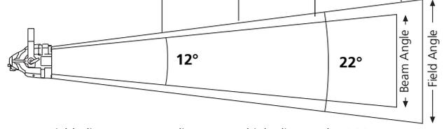
For Field diameter at any distance, multiply distance by 0.33
