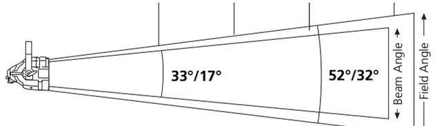
For Field diameter at any distance, multiply distance by 0.87/0.57
