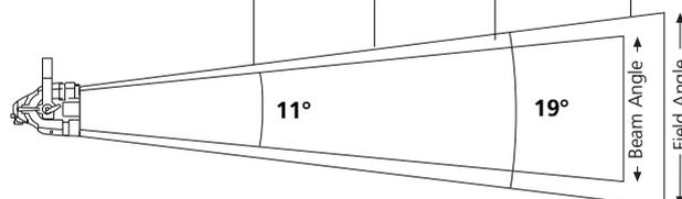
For Field diameter at any distance, multiply distance by 0.31
