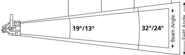
For Field diameter at any distance, multiply distance by 0.57/0.41
