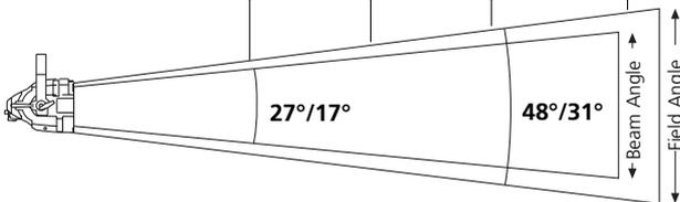
For Field diameter at any distance, multiply distance by 0.89/0.56
