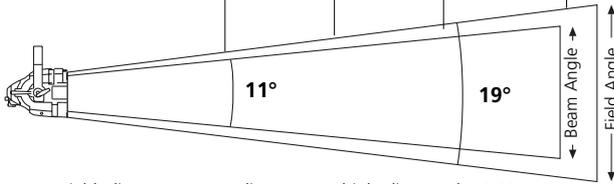
For Field diameter at any distance, multiply distance by 0.33
