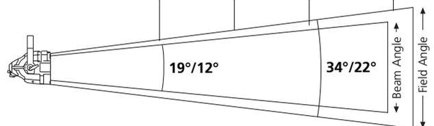
For Field diameter at any distance, multiply distance by 0.55/0.39
