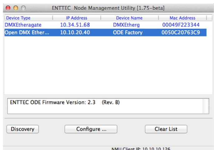
6. Once found, ODE will appear in the device list, with it's IP address and configured name. Select the ODE and click on configure button to get to the Configure ODE window, from where most of the settings can be changed.
