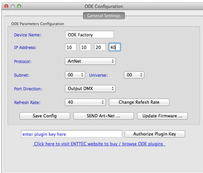
7. At your option, you may choose to enter a new name for the ODE in the Device Name field. Calling it "Truss 1" or "Onstage Dimmers Universe" may be convenient to your application, for instance.
